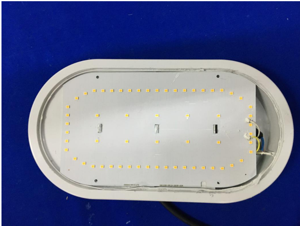
Figure 11. Internal view of MT60180
