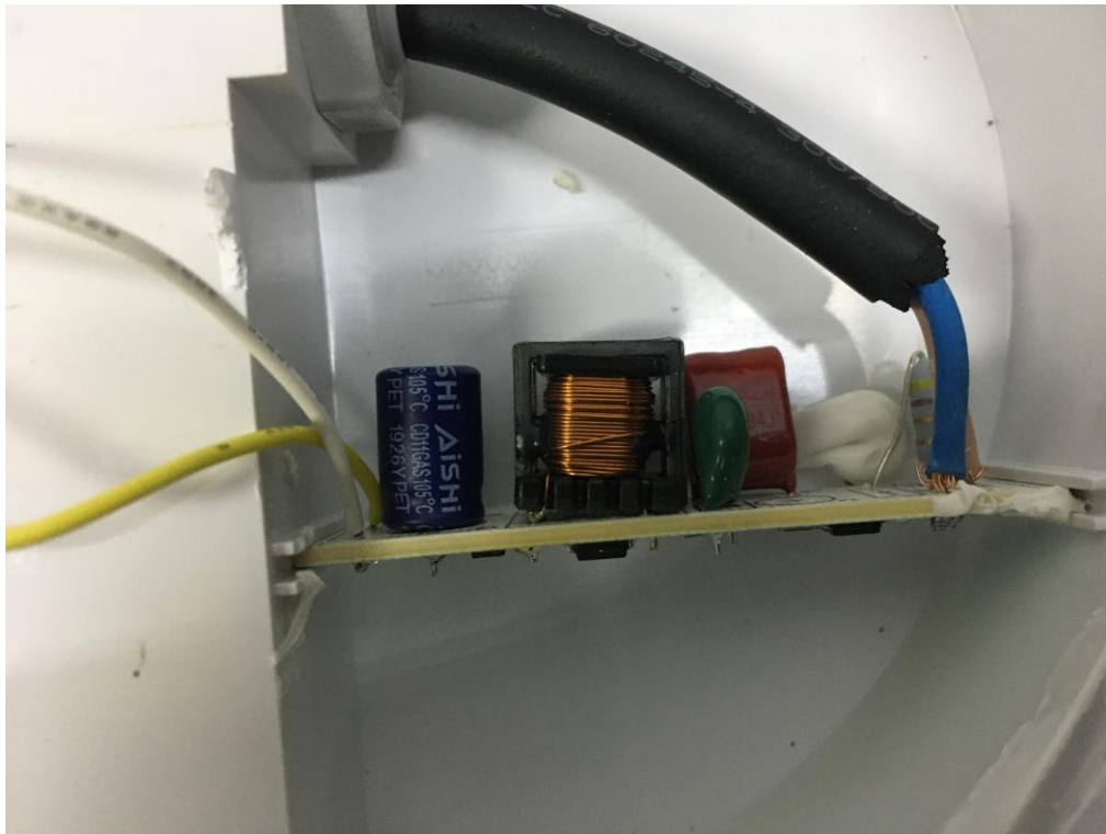
Figure 13. Internal view of MT60180
