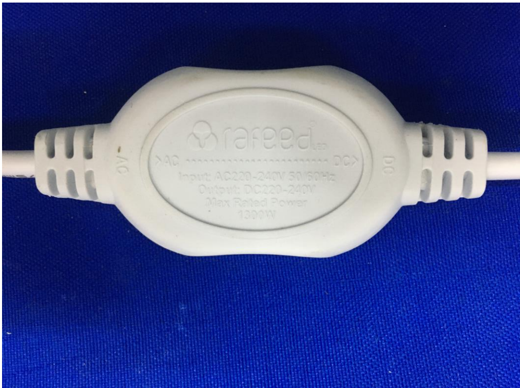
Figure 8 Over view of rectifier bridge
