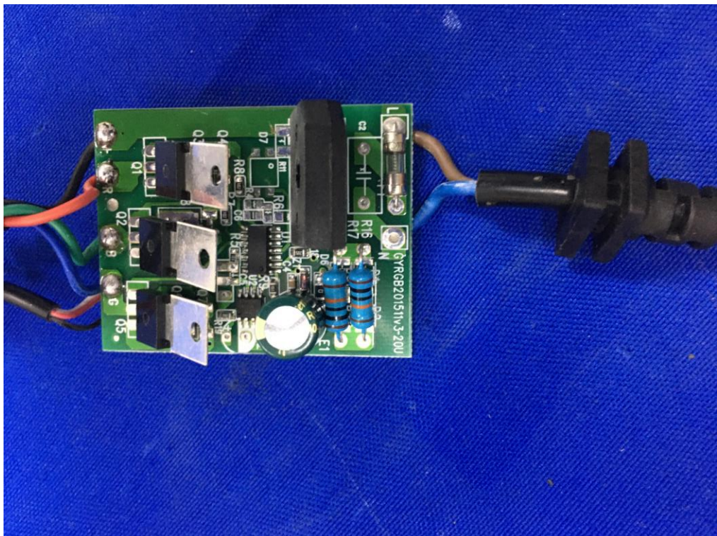
Figure 16 PCB view of rectifier bridge for RGB
