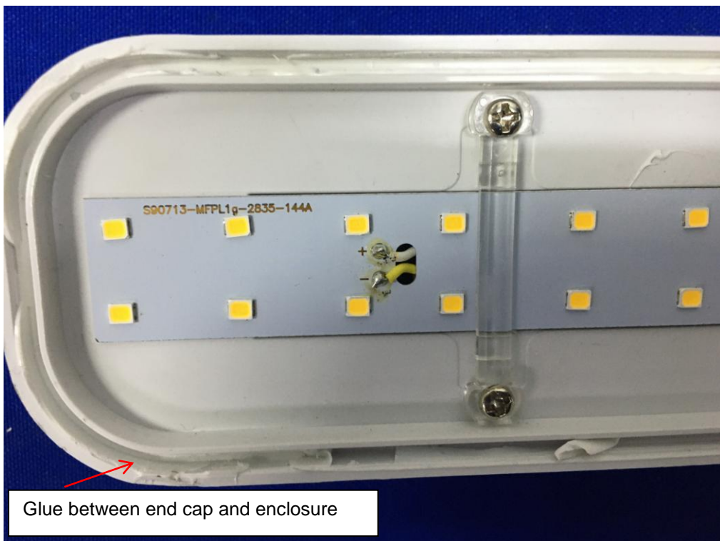
Figure 6. Internal view of model BH60190
